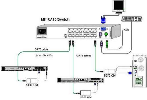
Figure 4 CAT5 KVM system connections
